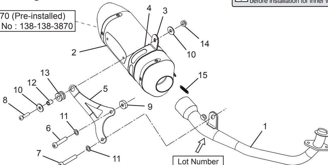
**! Note and record the weight of silencer assy before installation for inner wool maintenance.**
